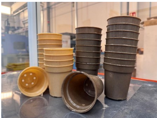
Planting pots with 1 mm wall thickness suitable for Green Wall design by AITIIP. Industrial injection moulding done by Techno Packaging using Wood K plus materials (@Photo: Techno Packaging)
